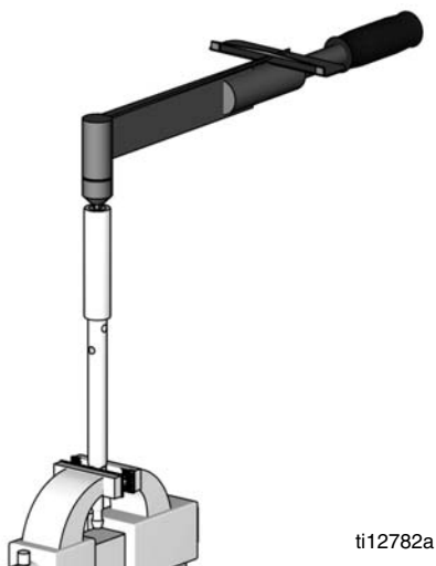
FIG. 2. Remove Flow-Through Nut
